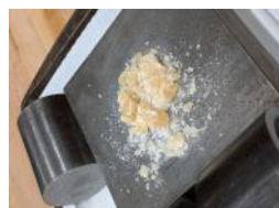
Fill remaining void with crushed stone, add CA glue, then hollow out inside.
