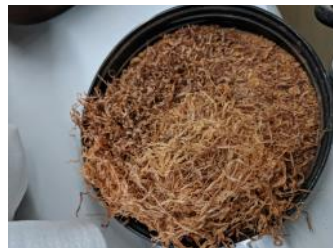
Pack voids with shavings leaving space near surface for crushed stone
